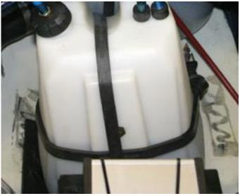
4. Use second strap and clip horizontally as in picture or into the grove on the tank. The second strap is slightly too long so you will need to tie a knot in this strap. <u>Both straps must be used</u>. Once into position, place original rubber retainer between tank and tray. Place a small piece of H/Turf between your Waterbox and new tank to prevent any rubbing.
