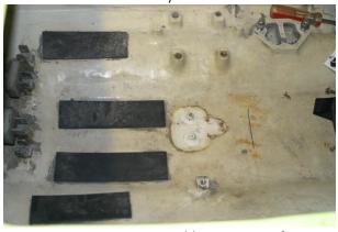
2. Place new battery tray into position using inner 2 original battery tray fixing points. Make sure all holes are clear of debris before tightening bolts supplied. You have been supplied 2 longer and 1 shorter bolt, the shorter bolt is for the side of the tray with only one fixing hole.
